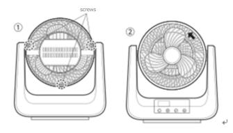
3. Twist the fan blade screw to the right and take the fan blade out, then you can clean the fan blade.
